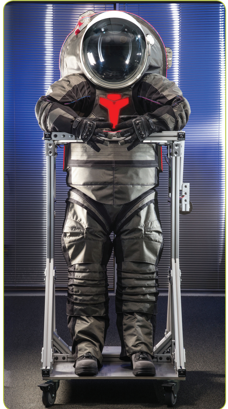
Above: A prototype of NASA's Z-2 spacesuit is pictured at the Johnson Space Center. Planned for use by astronauts as they travel to new deep-space locations, the suit incorporates a number of technology advances to shorten preparation time, improve safety, and boost astronaut capabilities during spacewalks and surface activities. (Oct. 14, 2015) PHOTO CREDIT: NASA
