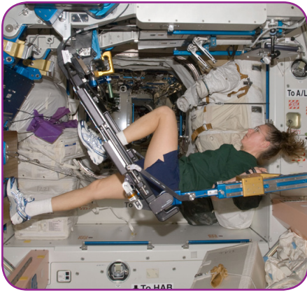
Above: Astronaut Sandra Magnus, Expedition 18 flight engineer, exercises on the advanced Resistive Exercise Device (aRED) in the Unity node of the ISS. PHOTO CREDIT: NASA
