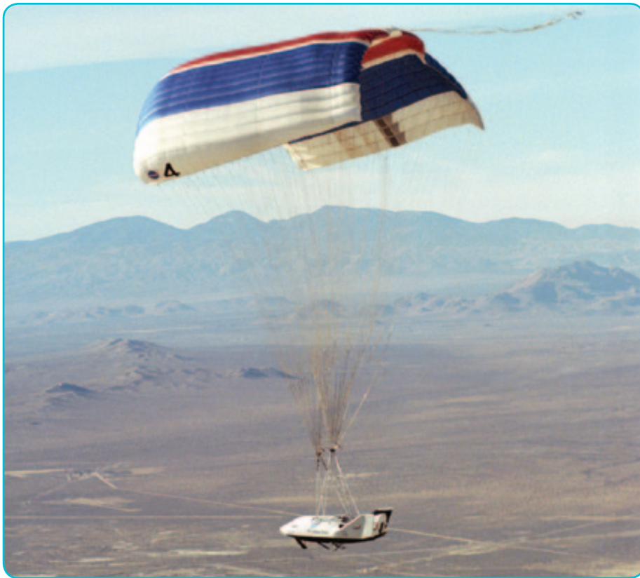
The X-38 prototype of the Crew Return Vehicle for the International Space Station undergoes a test with its 7,500-square-foot parafoil.
