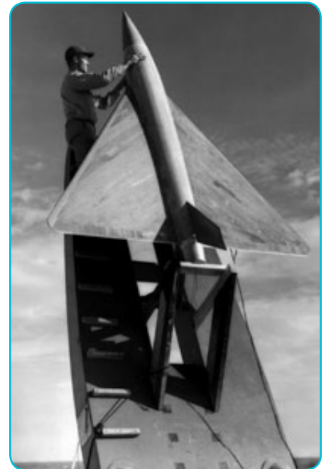
E17 Drag Research Model – On September 8, 1950, a technician prepares to measure the forces of thrust and drag on the flight of a research model.
